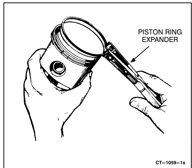
FIGURE 10-22. REMOVING PISTON RINGS
